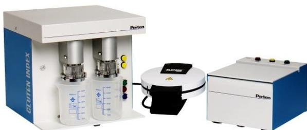
Glutomatic apparatus for gluten extraction
